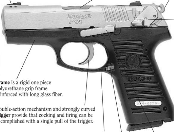
When ambidextrous **manual safety** is in "safe" position, the firing pin is cammed forward into the slide. This simultaneously places the firing pin out of reach of the hammer and locks the firing pin in a neutral position, preventing the firing pin from movement toward the cartridge. Further, the entire firing mechanism is completely disengaged from trigger.
