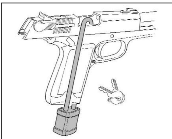
***Correct Installation of Lock
