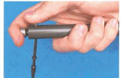
spring tube so that the lock tab is at the top of the bolt carrier. Insert the carrier from the rear of the receiver, be sure not to twist the bolt tube or push in the bolt as you insert it. Align the operating handle hole in the carrier with the cut-out in the receiver and insert the operating handle. Push the carrier up slightly so that the operating handle aligns with the slot for it and the recoil spring tube is parallel with the barrel of the pistol.
