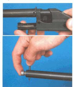
recoil spring and onto the piston rod. Insert the firing pin or similar tool into the piston head hole to temporarily hold the piston head in place. While slowly pulling out the firing pin, push in the piston pin from the other side until it is flush with the piston head. Twist the recoil spring tube so that the locking tab points towards the top of the bolt carrier. Check the operation of the recoil spring by lightly pulling on the recoil spring tube to compress the spring.
