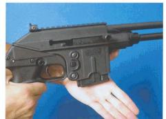
With the pistol's safety engaged, hold the pistol in one hand with the muzzle pointing in a safe direction and with your finger off the trigger and outside the trigger guard. Insert the loaded magazine into the grip until it is locked in place. Check to assure that the magazine is secure. Pull the operating handle back and release. This strips a round from the magazine and seats it in the barrel chamber.
