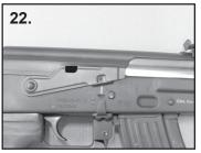
**Trigger:** Located in the trigger guard with safety disengaged and trigger pulled to the rear the firearm will discharge. **SEE FIG 27**
