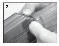
**Fig 2:** Depress the Upper Receiver Release Latch button and then depress the latch
