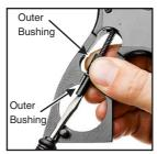
To adjust the hammer tension, remove the grip by loosening the single screw on the bottom of the grip and pulling it free from the frame. The adjustment knob is in the Frame. Use a small flat bladed screw driver to hold the inner bushing and turn the outer bushing to adjust. Turn clockwise to loosen the tension and counterclockwise to tighten. The tension can be checked by verifying that the firearm is unloaded, pointing the muzzle in a safe direction and "dry-firing" the revolver.
