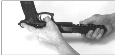
Figure 13 - Correct Position for Holding Slide for Reassembly
