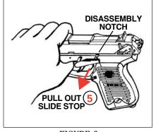
**FIGURE 6** Slide stop in disassembly position.
