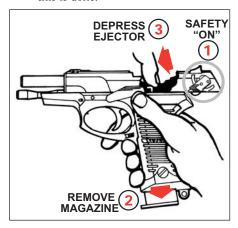
**FIGURE 4** Press slide stop up. Depress ejector.
