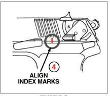
**FIGURE 5** Index marks aligned.
