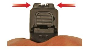
NOTE When pressing the sight, use a non-marring material against the sight and the slide to avoid damage to either.
