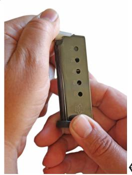
Insert the magazine into the magazine well at the base of the grip. Push until the magazine catch is fully engaged.
