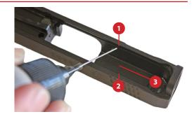
There are two lubrication points on the grip assembly. They are illustrated in the picture to the right.
