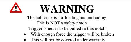
See explanation of how to put the firearm on half cock and also how to release from half cock at page 9 of this manual.
