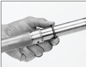
The tapered end of the gas bracket seal must face the gas bracket.
