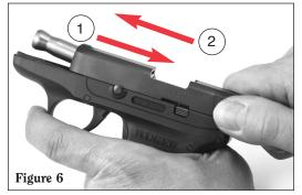
5. Push the slide backward slightly (1/16" or more) and pry loose the takedown pin using a screwdriver or other flat, blunt tool (see Figure 7).
