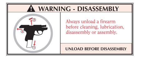
1. Keep pistol pointed in a safe direction. Press the magazine latch and withdraw the magazine from butt of pistol (see Figure 3).
