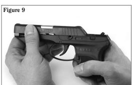
8. Compress the recoil spring assembly slightly to disengage it from its seat against the barrel lug, and remove it completely (see Figure 10).
