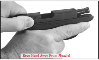
**Figure 2** Retracting the Slide
