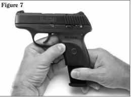
Pull slide to the rear and lock in the open position by pushing upward on the slide hold open. (See Figure 8)
