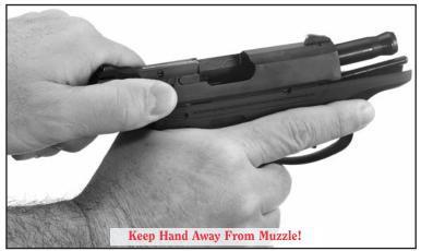
Figure 6 Retracting the slide.
