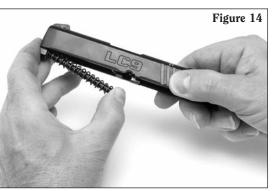
9. Remove the barrel. It will be necessary to move the barrel forward slightly and then down and back to extract it from the slide (see Figure 15).
