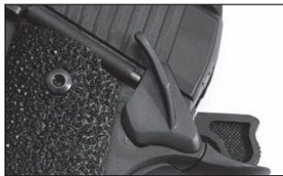
Figure 2: Thumb safety engaged
