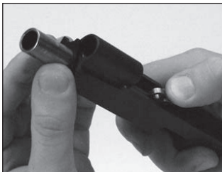
Figure 11: Insert barrel into slide
