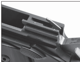
Figure 14: Plunger lever in the up position.
