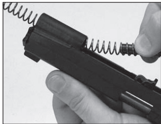
Figure 8: Removing recoil spring and guide
