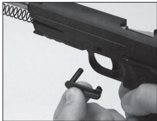
Figure 7: Removing slide stop
