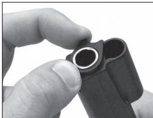
Figure 9: Removing bushing from slide
