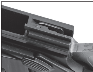
Figure 13: Plunger lever in the down position ready for assembly.
