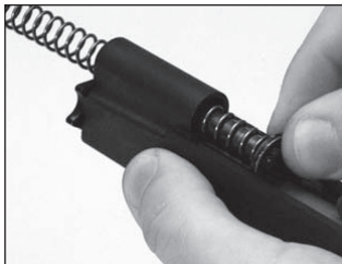
Figure 12: Insert recoil spring and guide into slide
