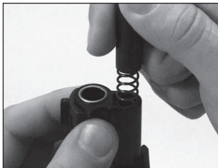
Figure 6: Releasing the recoil spring
