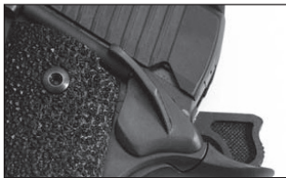
Figure 3: Thumb safety disengaged
