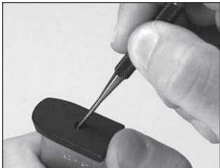
Figure 15: Field stripping the magazine
