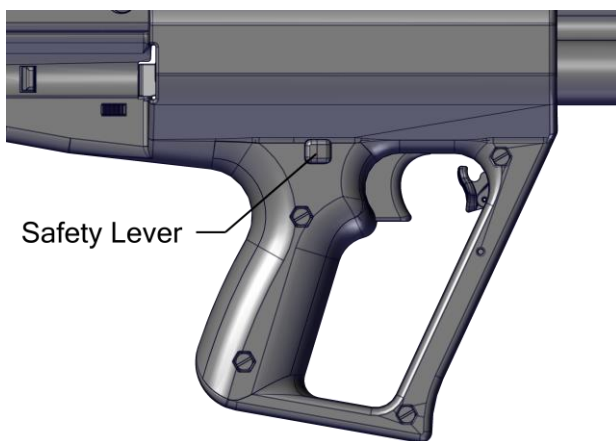
Figure 6-3 – TS12 Shotgun – Safety Lever Position
