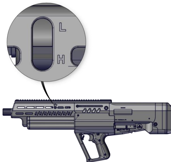
Figure 6-4 – TS12 Shotgun – Gas Cylinder Adjustment Lever Settings
