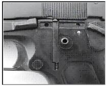
After the plunger tube assembly is removed, the slide safety may be removed, use care not to lose the slide safety tension spring. Assemble the left grip assembly in reverse manner and insure that both the thumb safety and slide safety are working correctly.
