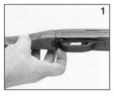
**DANGER:** The gun will fire when the trigger is pulled intentionally or acciddentally when the **RED BAND MARKING IS SHOWING.**
