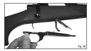
2. Prepare Axiom Rifle Stock for Installation by removing rear butt stock. To remove pull down on lever assembly and slide off buttstock. (Fig. 2)
