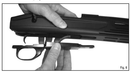
7. While holding the trigger guard and hinged magazine floor plate assembly in position, reinstall the two stock bolts removed in Step 1. (Fig. 7) Note: Take extra precaution not to cross thread bolts. For best performance, utilize a torque wrench and tighten bolts to a recommended torque of 65 inch lbs. Floor plate should open and close easily.
