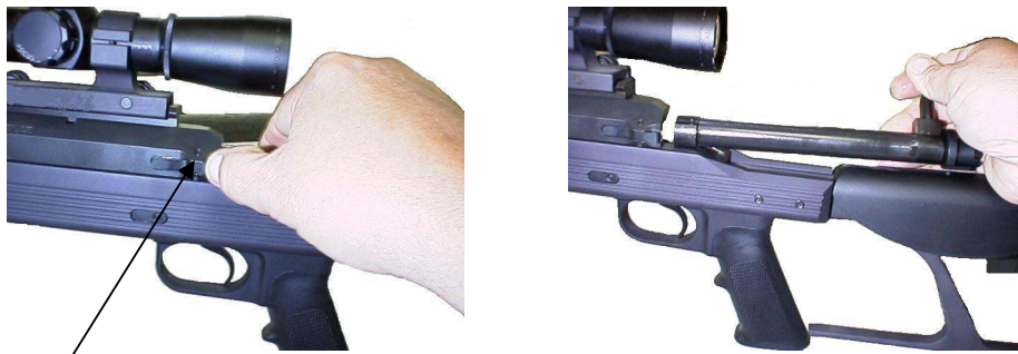
Figures 8 and 9 Removing the Bolt Assembly
