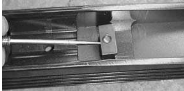
Figure 10 Loosening the Bedding Wedge
