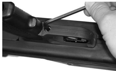
Figure 11 Removing the Grip Frame
