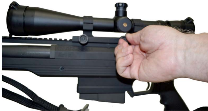
Attaching the ArmaLite® Scope Mount
