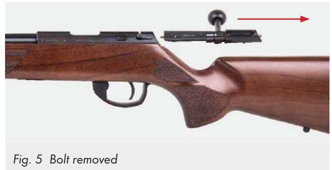
Fig. 4 Open and remove bolt
