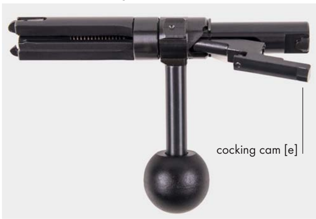
Fig. 32 Remove cocking cam [e]
