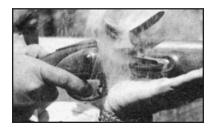
This Brown Bess was heavily primed and the resulting eruption has seriously distracted the shooter. Remember—use a light priming charge and wear safety glasses for extra confidence and protection.
