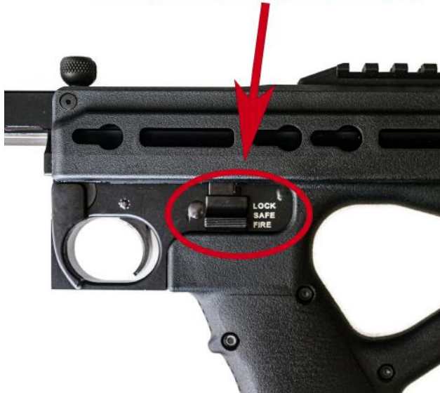
Figure 2. The left side of the trigger guard section of the rifle. In this illustration the safety is shown in the “lock” position. It should be in the “fire” position only when you are actually firing at a target.
