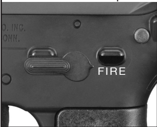
fig. 10 Manual safety in “FIRE” position
