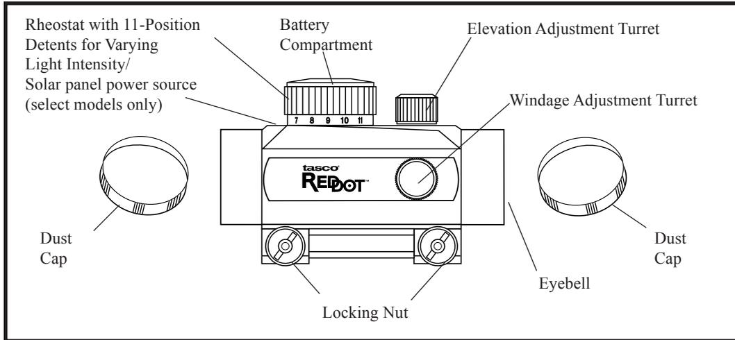
Congratulations on purchasing your Tasco Red Dot illuminated optical sight. Designed with a unique rheostat that features 11 positive detents for a full range of light intensities, this is a state-of-the-art scope designed for hunting, plinking and target shooting with pistols, rifles, shotguns and bows.
