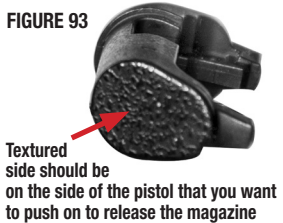
Magazine catch plunger on right side
