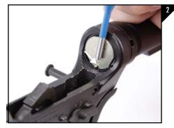
Using a punch, depress the buffer retainer spring as seen in Figure 2 and than remove the sring. When removing the spring be careful as the spring is under heavy tension.
