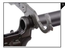
Hand tighten the castle nut to hold the locking ring in place, then take the AR tool and tighten the castle nut until tight as seen in Figure
