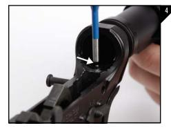
Using a punch, depress the buffer retainer pin as seen in Figure 4 and begin to unscrew the existing buffer tube.
