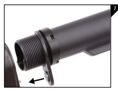
Place the lock plate onto the buffer tube, making sure the extended end is facing towards the weapon as seen in Figure 7.
