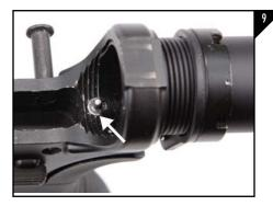
With your punch, depress the buffer retainer pin and make one more full rotation of the buffer tube until the buffer retainer pin sits into the grove on the buffer tube as seen in Figure 9. NOTE: For milspec installation there will be no groove on the tube, instead insure the tube covers the flat portion of the buffer retainer.
