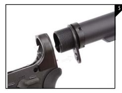
Once the tube clears the buffer retainer pin you may than finish unscrewing and remove the buffer tube leaving the pin in place as seen in Figure 5.
