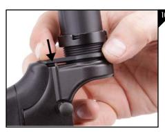
Next, press the locking ring tight to the lower receiver ensuring that the take down spring is properly seated as seen in Figure 10.
