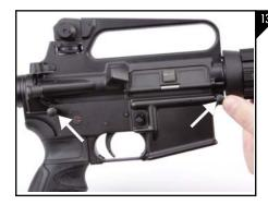
Reconnect the lower receiver to the upper receiver and push the rear and front take pins back into place as seen in Figure 13
