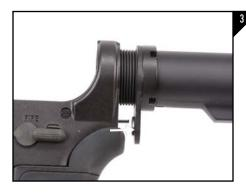
Next, using an AR tool, loosen the existing castle nut and slide the locking ring to the rear as seen in Figure 3. When sliding the lockng ring keep in mind that the spring for the rear take down pin is under tension.
