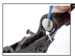
Reinstall the buffer and spring into the buffer tube until the spring is seated behind the buffer retainer pin as seen in Figure 12.
