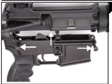
Begin by depressing and removing the front and rear take down pins and than detaching the lower and upper receiver as seen in Figure 1.
