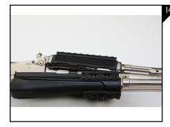
Install the gas tube into the gas piston. Next, align the upper handguard with the lower handguard and press the rear of the gas tube down until the lever can be locked as seen in Figure 14.
