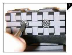
Using the provided 6-32 x 1/2" machine screws and a phillips head screw driver tighten the rails to the handguard as seen in Figure 9.
