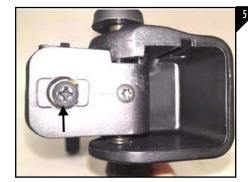
With the stock in the folded position slide the buffer tube into the pivot housing. Using the provided 14 x 1 1/4" phillips head plastite screw and a phillips head screwdriver, tighten the buffer tube to the pivot housing as seen in Figure
