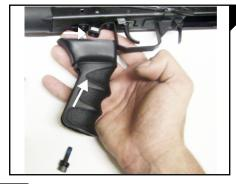
Install the new ATI pistol grip by holding the supplied pistol grip T-nut onto the pistol grip mount bracket. Now, slide the pistol grip and the M6 x 1 x 25mm into place behind the trigger guard. Use a 5mm allen wrench to fasten the pistol grip bolt to the pistol grip nut on the mount bracket as seen in Figure 6.
