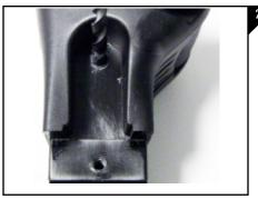
If the screw measures .230 remove the pivot assembly and start by drilling pilot holes in the center of the 2 marked holes with a 1/16" starter drill bit as seen in Figure 2. Next, move up to the 3/16" drill bit and drill 2 wider holes using the two pilot holes.
