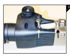
Place the pivot housing assembly into the receiver, insert the (2) original screws and tighten both screws to secure the stock to the receiver as seen in Figure 3.
