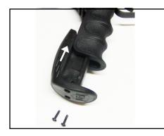
Insert the scorpion recoil pad onto the back of the pistol grip and secure using the provided (2) 6 x 48/2 x 1/2" plastite screws and a phillips head screwdriver as seen in Figure 7.
