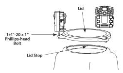
Install **lid** by aligning handles with notches in **hopper top**. Twist until lid rests flush against **lid stop**.
