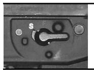
Keep the safety "ON" unless actually firing. Always move the safety to its intended position and check it. The safety is not "ON" unless it is completely "ON." Never depend on a safety mechanism or any other mechanical device to justify careless handling or permitting the rifle to point in an unsafe direction. The only "safe" rifle is one in which the bolt is open, the chamber is empty, and there is no magazine in the gun.
