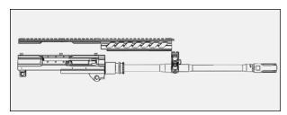
STEP 10 REMOVAL OF UPPER RAIL SECTION
