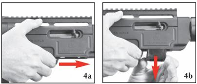
**Figure 4.** The safety should be "on" when the magazine is being removed or inserted. Move the magazine release forward (Figure 4a) and draw the magazine out by grasping it between your thumb and forefinger and draw it out of the gun (Figure 4b).
