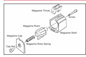
Exploded view of the SR-22 magazine components. This illustration is included to show the relationship and names of the magazine components. As noted in the text above, the magazine should not be disassembled.
