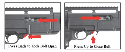
To release the bolt: Retract the bolt handle to its extreme rearward position and then press in on the upper section of the bolt lock. Release the bolt and it will move fully forward.
