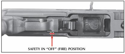
**Figure 3.** The underside of the trigger guard section of the rifle. In this illustration the safety is shown in the "off" (fire) position. The position of the safety and red band indicate the safety is "off." It should be in this position <u>only</u> when you are actually firing at a target.
