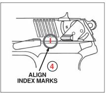
Figure 7 Index marks aligned.
