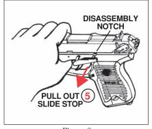
Figure 8 Slide stop in disassembly position.
