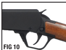
FIG 10 Hammer in the safety (half cocked) position
