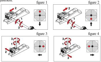
To raise or lower the sighting, first loosen the lateral screw on rear sight. To raise the sight, adjust according to the steps in figure 1.
