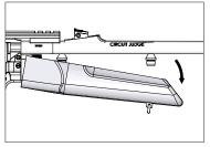
Keeping the cylinder open according to the figure 5, press the CYLINDER CATCH, and then remove the cylinder set.
