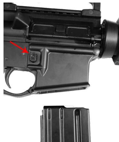
4. Remove the ammunition source by removing the magazine. To do so, depress the magazine release button and pull the magazine out the bottom of the magazine well.
