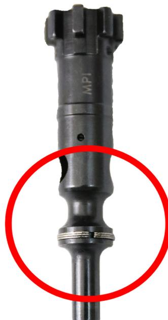
Incorrectly Staggered Gas Rings
