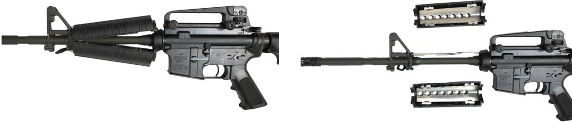
With the handguards out of the way, be certain not to distort or damage the gas tube.
