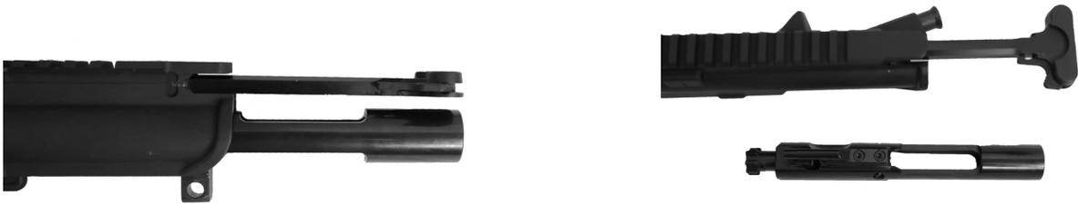
7. Remove the charging handle by sliding the charging handle to the point where the “ears” (or protruding tabs) on the charging handle can slip through the keyway on the upper receiver. When the charging handle is extended out approximately 4.4” from the upper receiver, the ears on the charging handle should be lined up and can slide up through the keyway.
