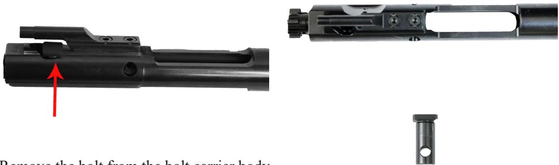
12. Remove the bolt from the bolt carrier body.
