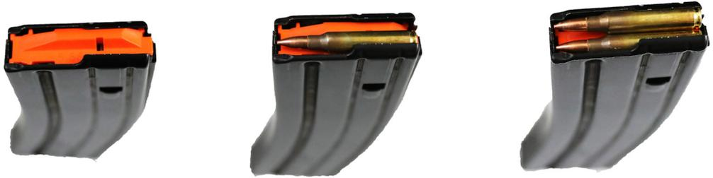
6. Repeat step five, placing additional rounds on top of each other in a staggered column, until the magazine is fully loaded.
