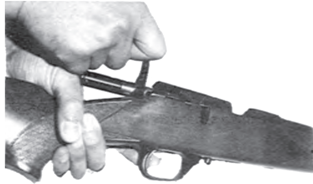
Fig. 10 Withdrawal of trigger and removal of bolt
