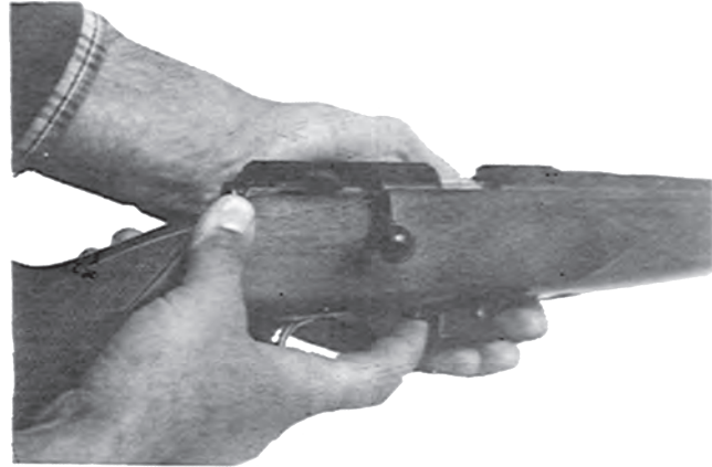
Fig. 9 Separation of magazine from rifle
