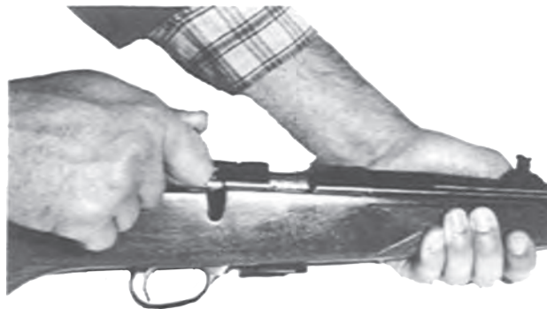
Fig. 13 Loading of rifle (cartridge inserting into barrel)
