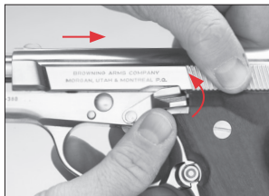
Move the slide rearward and push in the slide release/stop latch to lock it rearward.
