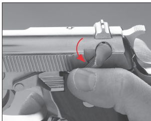
Slide the “safety”/decocking lever down to decock the hammer.
