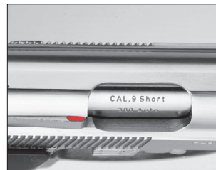
The protruding extractor (with red index mark) confirms that a cartridge is present in the chamber.
