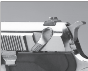
The “safety”/decocking lever in the on safe position.
