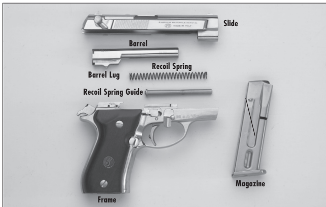
Disassembly to this point is sufficient for normal maintenance of your pistol.
