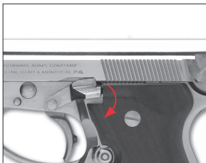
Depress the slide release/stop latch.
