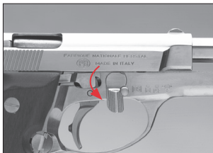
Rotate take-down lever counterclockwise 90 degrees downward.
