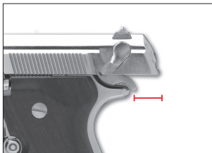
The slide moves rearward about \frac{3}{4} " past the end of the frame.
