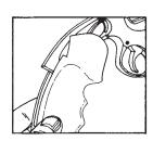
MONOGRIP should be guided up behind the trigger guard, then pivoted to cover the frame straps. The grip must mate with the semi-circular "loops" at the top of the firearm handle. MONOGRIP must be fully seated on the frame before inserting mounting screw.
