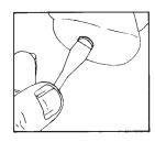
Insert the screw so it enters the stirrup threads and using an appropriate screwdriver, tighten the screw until snug, no tighter. Over-tightening does nothing to increase grip tightness and can damage the screw or stirrup.
