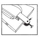
When in place, the stirrup is a clamp that provides a screw thread hanging below the handle for securing MONOGRIP to the frame. No alteration of the firearm frame is needed. Remove screw from put
