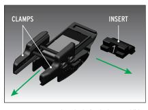
Turn screws counter clockwise to loosen. Slide clamps away from Insert. Remove Insert #1 by sliding to the right.
