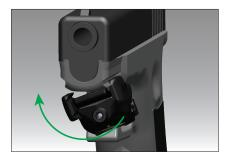
Attach Rail Master at desired location on firearm rail and rotate into place, aligning insert with rail lug. Turn screws clockwise to secure clamps to rail.
