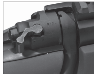
“Safety” shown in the on safe position.
