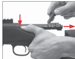
Press the bolt stop and pull the bolt rearward, out of the receiver.
