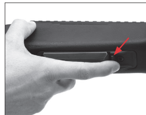
Press the magazine release.
