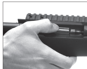
Press the cartridge down until it snaps into place.
