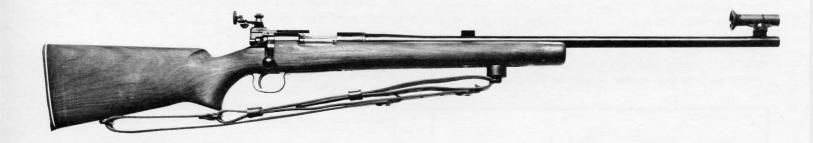
The Remington "Rangemaster" Model 40X is a bolt action 22 caliber match rifle. This rifle is of single shot solid frame design chambered for long rifle cartridge only. The gun action is hand operated and similar in function with most rifles of the bolt action type. Also included in this supplement is the Model 40XR. Unless otherwise specified, instructions are same as for the Model 40X.
