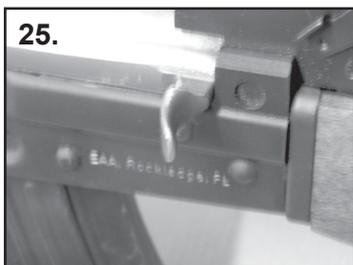
the magazine well. With the lugs engaged you should be able to swing the magazine up into the locked position. To remove the magazine push the magazine release lever forward and swing the magazine down while pushing the magazine release lever. **SEE FIG 26**
