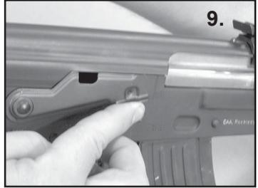
7. **Fig 9:** After determining there are no obstructions in the chamber release the bolt and move the bolt block safety up or in the safe position, so that it blocks the movement of the bolt.
