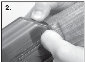
**Fig 2:** Depress the Upper Receiver Release Latch button and then depress the latch
