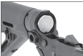
FIG 42 BUFFER HELD INTO RECEIVER EXTENSION
