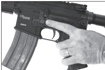
FIG 25 MAG CATCH BEING DEPRESSED LEFT AND RIGHT SIDE
