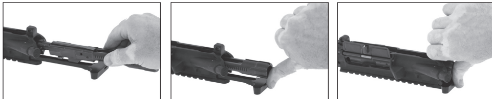
FIG 47 REINSTALLATION OF THE BOLT CARRIER ASSEMBLY TO UPPER RECEIVER
