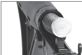
FIG 41 ACTION SPRING AND BUFFER STARTED INTO RECEIVER EXTENSION
