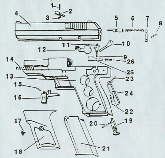
Safety/Slide Lock is located at top of left grip. Sliding safety lever upward, into slide notch engages safety, exposes letter (S) on grip and places pistol in "SAFE" position.
