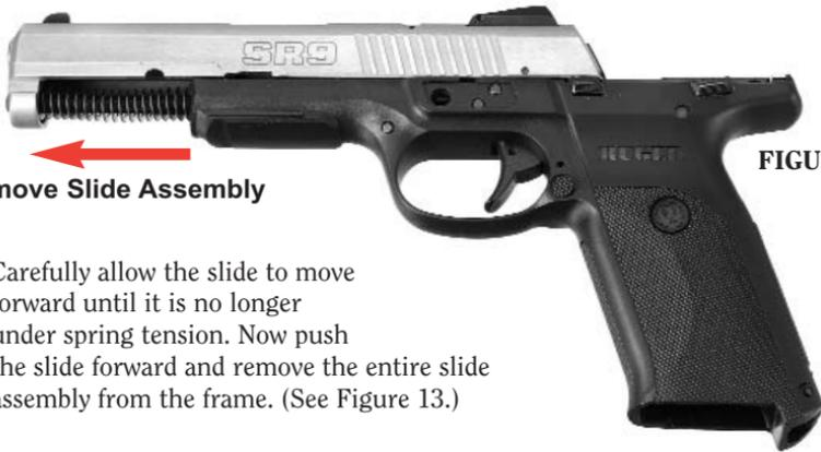
5. Carefully allow the slide to move forward until it is no longer under spring tension. Now push the slide forward and remove the entire slide assembly from the frame. (See Figure 13.)
