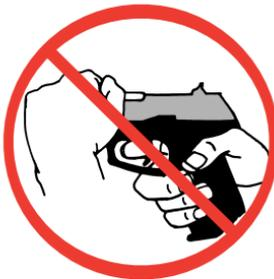
The slide should always be pulled rearward (“retracted”) by pulling the rear portion of the slide in the vicinity of the serrations. **Always keep fingers away from trigger!**
