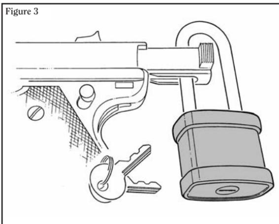
***Correct Installation of Lock For
