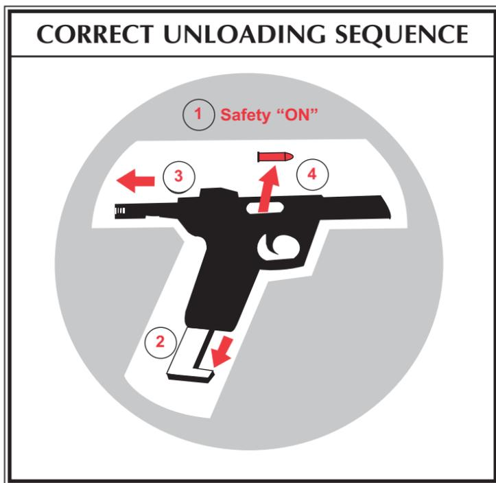
4. If desired, the bolt can be left in the open position, being held there by the bolt stop. If it is desired to close the bolt, again look to be certain the chamber is empty. Assuming that the magazine is not in the pistol and that the safety is “on” (S), retract the bolt to its rearmost position, release it, and the bolt will snap forward (on Mark III models). On 22/45 models the bolt stop button must be depressed. Keep your fingers out of the receiver!
