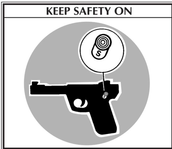
8. The pistol is ready for instant use once the safety is disengaged. Firing will automatically reload and recock the pistol. **Note that every time the trigger is pulled, if a cartridge is in the chamber and the safety is “off,” the pistol will fire — be careful!**
