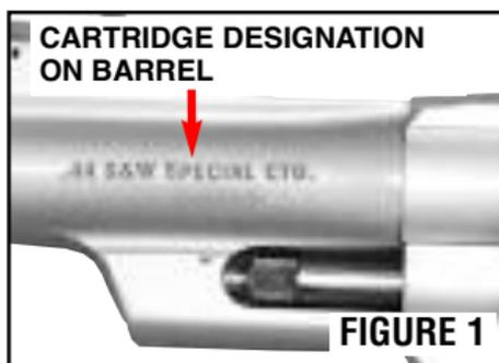
Never use a cartridge not specifically designated for use in your firearm. The wrong type of ammunition may exceed the capability of your firearm and may damage or even rupture your firearm.
