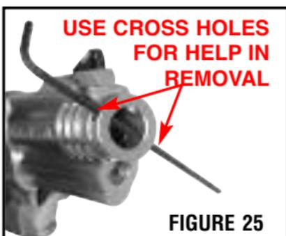
3. Remove the compensator from the barrel for cleaning or for a compensator change. (Figure 26)
