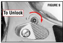
position on revolvers with exposed hammers. A definite stop and detent will be felt when the key is turned to either the locked or the unlocked position. (Figure 9)
