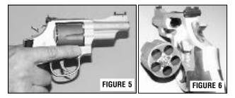
When you inspect your revolver, you must first check for yourself to ensure that it is unloaded. Do this with your finger off the trigger and out of the trigger guard (Figure 5) and keep the barrel of the firearm pointed in a safe direction. Press the thumbpiece forward and push the cylinder to the left (Figure 6).
