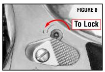
The key will turn approximately 90°. The locked indicator flag will become visible on revolvers with exposed hammers. A definite stop and detent will be felt when the key is turned to either the locked or the unlocked position. (Figure 8)
