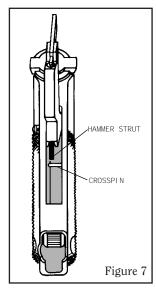
If you cannot place the hammer in the horizontal position, it is most likely because the hammer strut is trapped behind the crosspin (see Figure 7 – not applicable to 22/45 models). If this occurs, lift the hammer to free the hammer strut from behind the crosspin and then move the hammer into the horizontal position.
