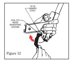
While holding the pistol in this position and depressing the trigger, move the mainspring housing into its proper place in the frame. (See Figure 13.)
