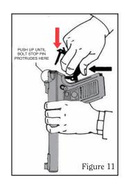
fully in place to close the latch in Step 8. Do not yet move the mainspring housing into the frame.
