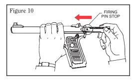
first time the trigger is pulled on an assembled pistol, the firing pin will fly forward so far as to irreparably dent the rear end of the chamber of the barrel, making the pistol useless. Now, slide the bolt (with the recoil spring upward) fully forward into the receiver. (See Figure 10.)
