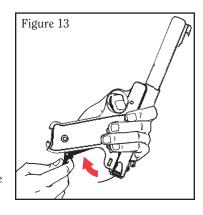
far as it will go without excessive pressure. Holding the mainspring housing in this position, release the trigger and remove the magazine. Once the magazine is removed, the mainspring housing will close the rest of the way.
