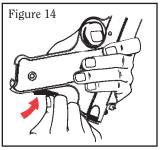
10. Replace <u>empty</u> magazine, point pistol in a safe direction and pull the trigger to uncock the gun. Guns should not be stored loaded or cocked. Note that in order for the internal lock to be engaged, the pistol must remain cocked, and the manual safety must be put "on" safe. (See p. 13.)
