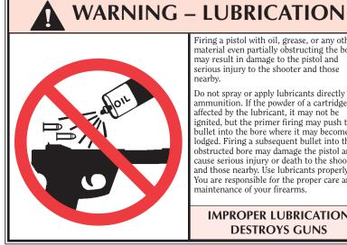
Firing a pistol with oil, grease, or any other material even partially obstructing the bore may result in damage to the pistol and
