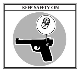
8. The pistol is ready for instant use once the safety is disengaged. Firing will automatically reload and recock the pistol. Note that every time the trigger is pulled, if a cartridge is in the chamber and the safety is "off," the pistol will fire — be careful!
