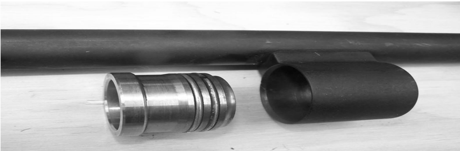
View Of Gas piston removed for cleaning.
