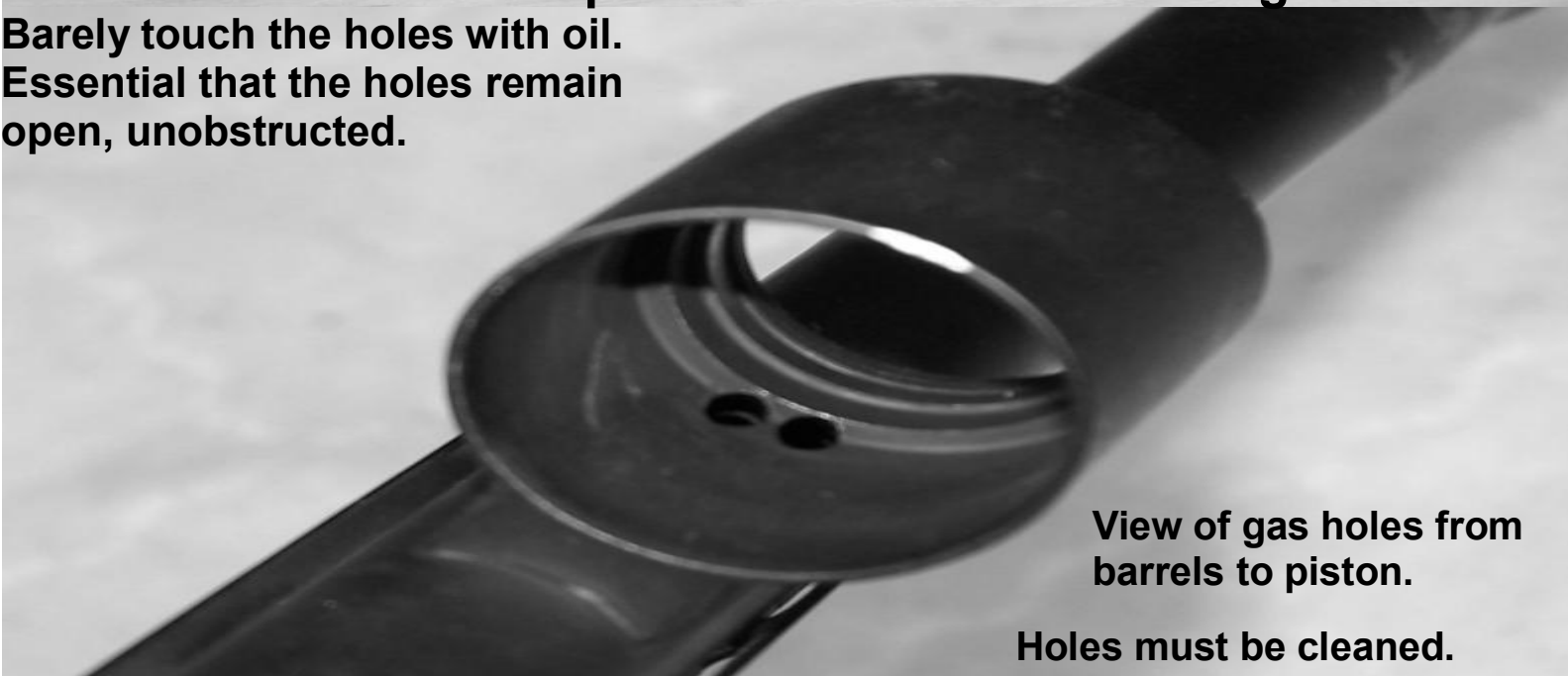
View Of Gas piston removed for cleaning.
