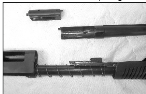
Auto bolt return action spring location
